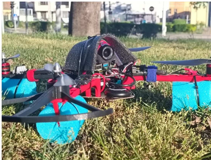
Fig. 1. Designed UAV platform with video streaming capabilities
